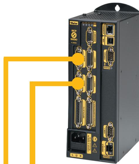
Analog +/- 10V signal for torque and velocity modes
