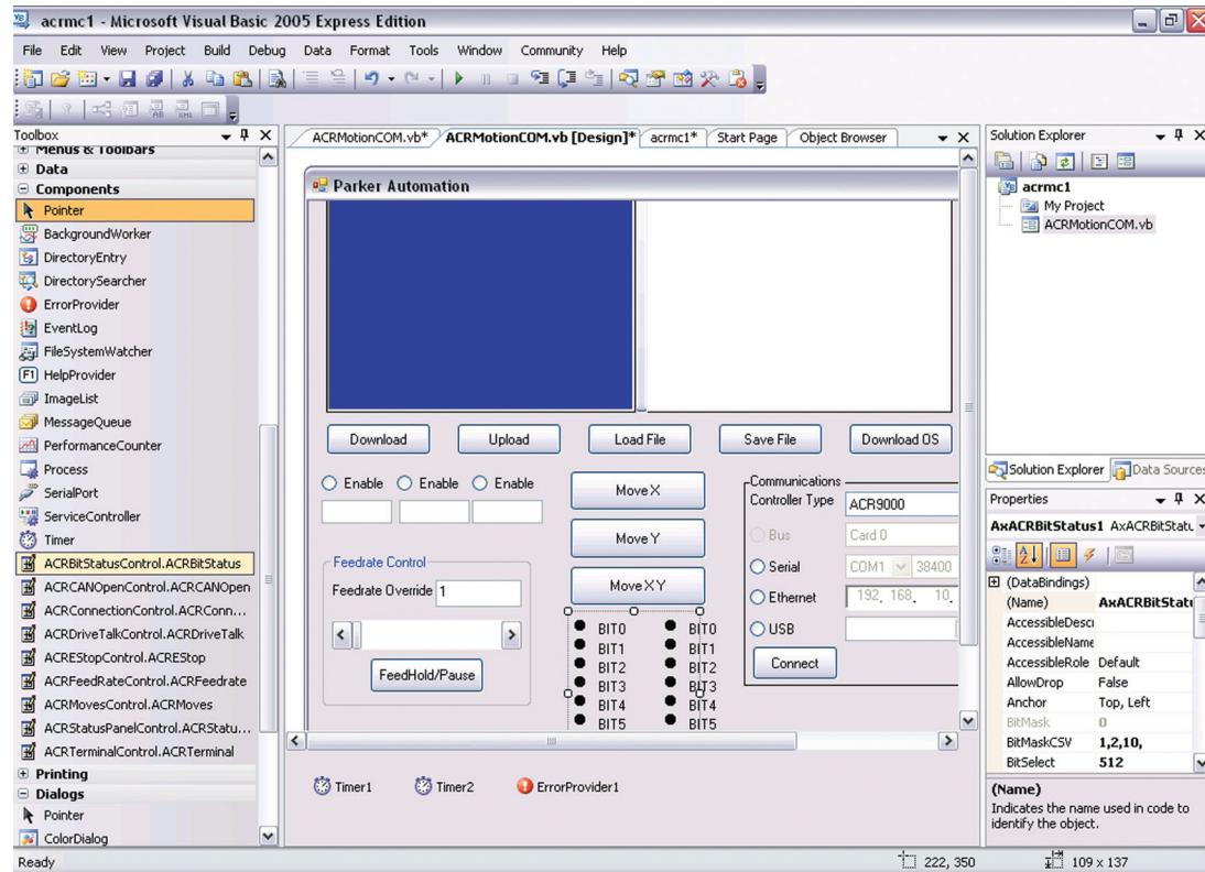
The ACR MotionCOMponents Tool Kit is an extensive collection of components and controls to allow a software developer to quickly and easily build a custom user interface for PC-based motion control applications. The tools incorporate a full set of ACR function calls, enabling complete control of any ACR family controller from a PC program.
