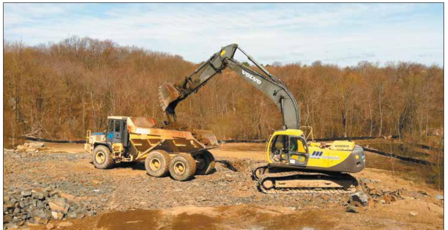
A Volvo excavator loads blasted rock into an off-highway hauler.
