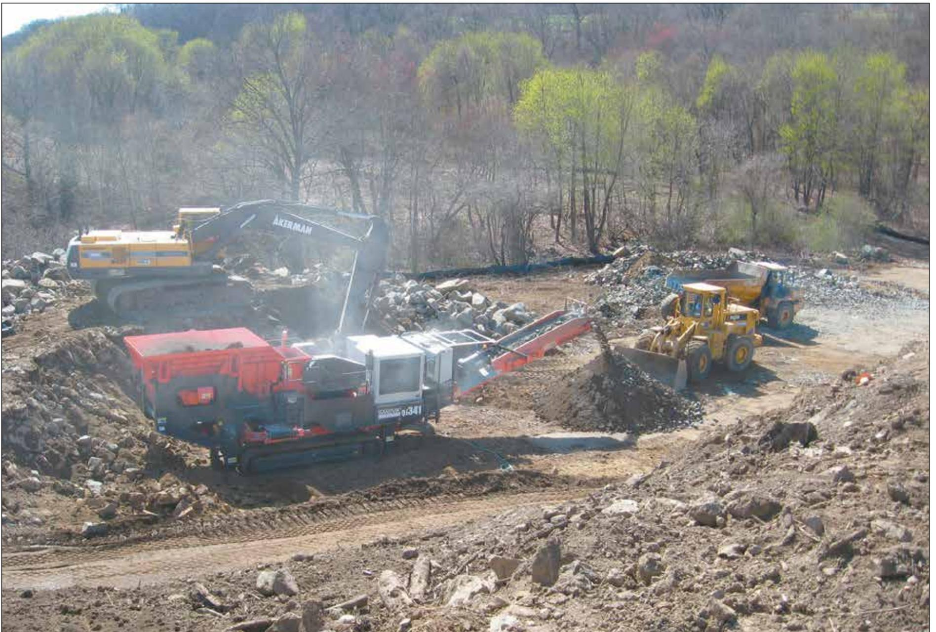
*An Akerman EC450 feeds blasted rock to Sandvik QJ341 Mobile Crusher while a Cat 950 Loader works to remove crushed material.*
