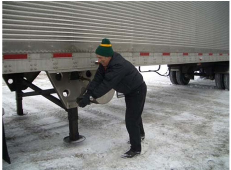
Figure 1 - Manual Cranking to lower the Trailer Landing Gear
