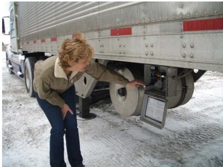
Figure 2 - Air activation allows the landing gear to be raised and lowered with a finger activated lever
