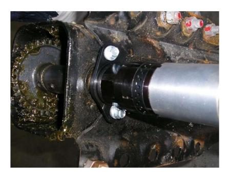
Motor shown attached to wing plate.
