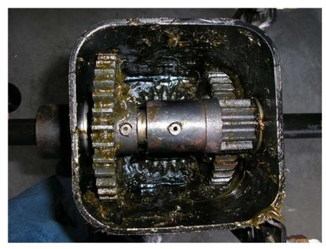
Jost drive leg show with access cover removed. Spur gear is shown on right of the top gear train.
