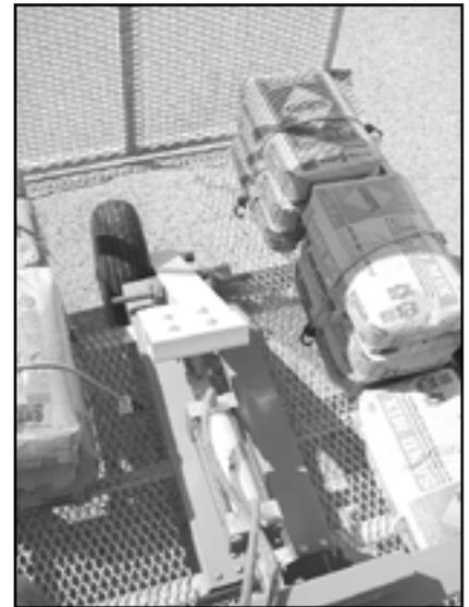
*Test rig, lower photo, consisted of a pneumatically actuated pivoting arm mounted on a trailer towed behind a pick-up truck.*
